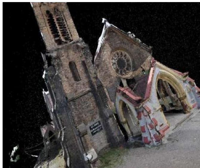
Fig. 3.8 Resultant point cloud of church after geo-registration
