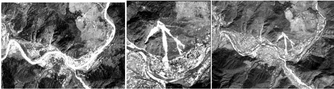
Fig. 1.15 IRS-PAN image of Uttarkashi before landslide, after landslide and PAN image
