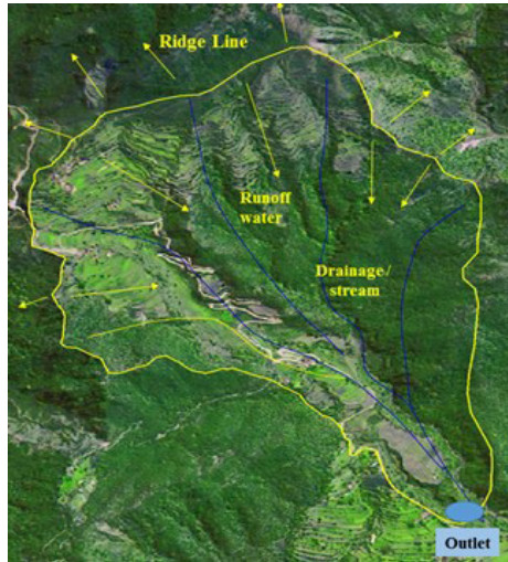
Fig 12.2. Watershed delineation with outlet showing ridge line & drainage lines on Natural Colour Composite of Resourcesat-1 LISS IV data
